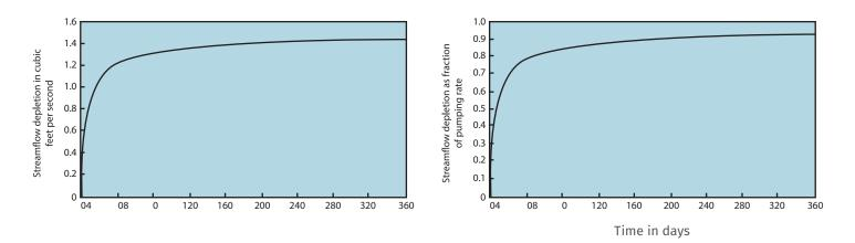
Figure B–1. Streamflow depletion resulting from pumping at a well located 250 feet from a stream. The well is pumped at a rate of 1 million gallons per day (about 1.55 cubic feet per second). In graph A, streamflow depletion is expressed as a rate, in cubic feet per second; in graph B, depletion is expressed as a fraction of the pumping rate at the well, which is a dimensionless quantity. (USGS Circular 1376)
