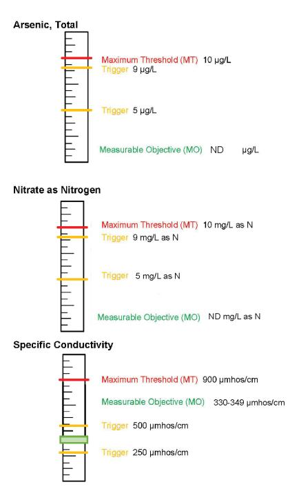
Figure 1.10: Visual Representation of the Sustainable Management Criteria of Arsenic, Nitrate, and Specific Conductivity for Well 4710001-003 of the Monitoring Network. Measurable objectives are specific to each well in the monitoring network. If the measurable objective is higher than one of the triggers, then that particular trigger is not applicable to that well.
