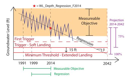
Figure 1.7: Visual description of the minimum threshold and soft landing trigger on a hydrograph.
