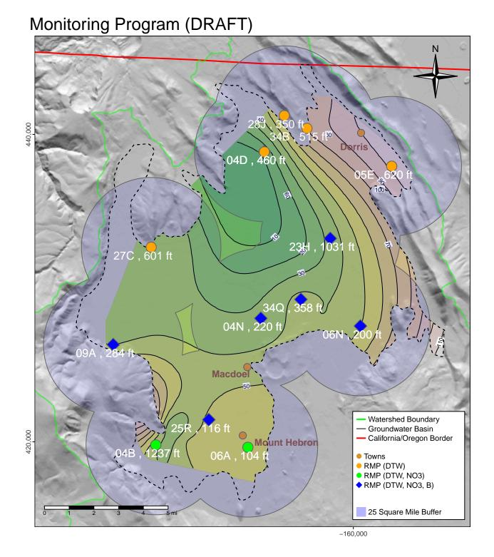
Figure 1.3: Representative monitoring points (RMP) in the water level and water quality monitoring networks. Yellow RMPs indicate wells dedicated to water level monitoring only. Green, blue, and red RMPs indicate water level and water quality sampling points. Well names corresponding to the shorthand names on the map are shown in Table 2. All water quality RMPs are also water level RMPs. In other words, the water quality monitoring network is a subset of the water level monitoring network.
