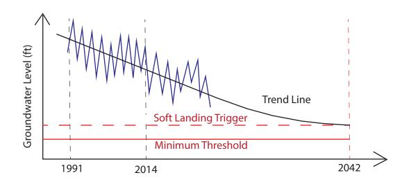
Figure 1.6: The goal for groundwater levels is to slow any decline down to the soft-landing trigger and no lower. The soft-landing trigger initiates strict management actions to prevent further decline to the minimum threshold.
