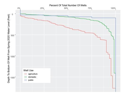
Figure 1.9: Number of wells in Butte Valley at a series of well depths. The deeper the MT is set, the more well outages occur and the higher the pumping cost.
