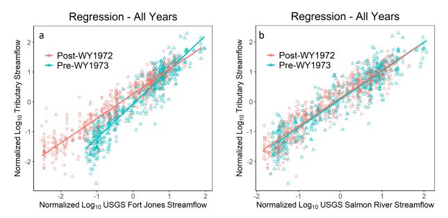
Figure 1. Scatterplot with linear regressions between gaged monthly flows in Scott River tributaries and gaged monthly flows in (a) Scott River USGS gage currently used in SVIHM, and (b) Salmon River at Somes Bar USGS gage which we recommend using for some sites and months. Colors differentiates the older WY 1957–1972 period from the more recent WY 1973–2016 period.
