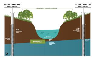
**Figure 6. Contouring depth-to-groundwater around surface water features and GDEs. (a)** Groundwater level interpolation using depth-to-groundwater data from monitoring wells. **(b)** Groundwater level interpolation using groundwater elevation data from monitoring wells and DEM data.
