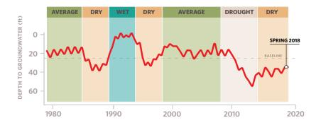
Figure 3. Example seasonality and interannual variability in depth-to-groundwater over time. Selecting one point in time, Spring 2018, characterize groundwater conditions in GDEs fails to capture what groundwater conditions are necessary to maintain ecosystem status into the future so adverse impacts are avoided.
