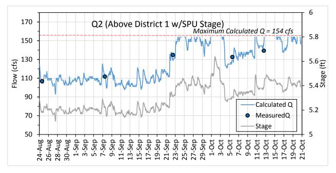
FIGURE 14. STAGE, MEASURED Q, AND CALCULATED FLOW (Q) FOR Q2 THROUGHOUT THE STUDY PERIOD. STAGE DATA RETRIEVED FROM CDEC (DWR STATION SPU).
