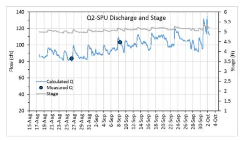
FIGURE 11. STAGE, MEASURED FLOW (Q), AND CALCULATED FLOW (Q) FOR Q2-SPU THROUGHOUT THE STUDY PERIOD: AUGUST 17TH THROUGH OCTOBER 3RD, 2016. FLOWS WERE LESS THAN THE MAXIMUM CALCULATED FLOW VALUE OF 140 CFS FOR THE ENTIRE STUDY PERIOD.
