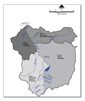
FIGURE 2. HYDROLOGICAL ZONES IN THE SHASTA BASIN BASED ON THE DOMINANT HYDROGRAPH COMPONENTS THAT DETERMINE RUNOFF PATTERNS IN THE MAINSTEM SHASTA RIVER. BOUNDARIES ARE APPROXIMATE. GRAPHIC FROM: (MCBAIN & TRUSH, INC ET AL. 2010).
