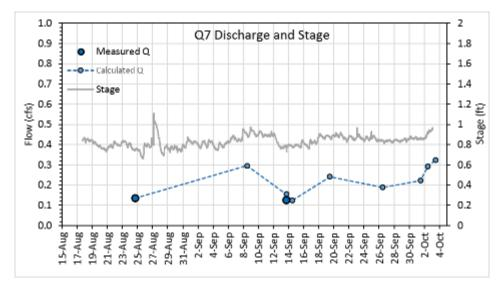
FIGURE 16. STAGE AND MEASURED FLOW (Q) FOR Q7 THROUGHOUT THE STUDY PERIOD: AUGUST 17TH THROUGH OCTOBER 4TH, 2016. A RATING WAS NOT DEVELOPED AT Q7 BECAUSE ONLY TWO MEASUREMENTS WERE PERFORMED. INSTEAD, THE CONFINED CHANNEL GEOMETRY AND VELOCITY MEASUREMENTS WERE USED TO CALCULATE FLOWS ON ASSESSMENT DAYS.
