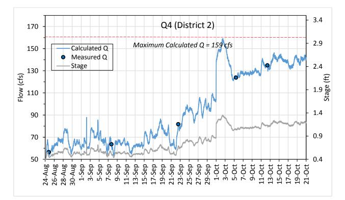
FIGURE 18. STAGE, MEASURED FLOW (Q), AND CALCULATED FLOW (Q) FOR Q4 THROUGHOUT THE STUDY PERIOD.
