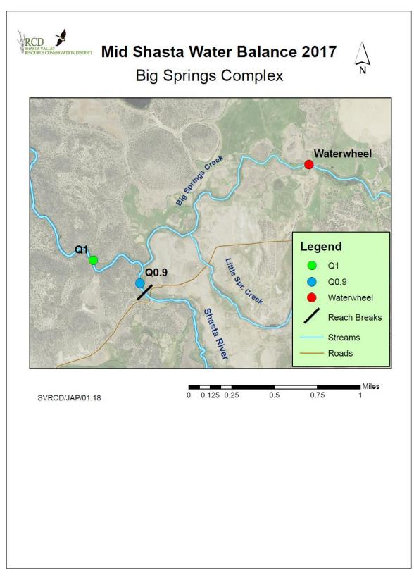
FIGURE 7. MAP OF THE BIG SPRINGS COMPLEX INCLUDING MEASUREMENT SITES AND "WATER WHEEL" EXISTING STAGE/DISCHARGE SITE ON BIG SPRINGS CREEK. ALSO IDENTIFIED IS LITTLE SPRINGS CREEK DOWNSTREAM OF THE WATER WHEEL SITE.
