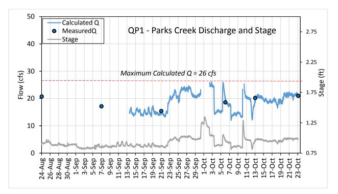
FIGURE 12. STAGE, MEASURED FLOW (Q), AND CALCULATED FLOW (Q) FOR QP1-PARKS CREEK ABOVE SHASTA RIVER CONFLUENCE, SEPTEMBER 24<sup>TH</sup> THROUGH OCTOBER 24<sup>TH</sup>, 2017. RATING PRIOR TO SEPTEMBER 24<sup>TH</sup> NOT USED DUE TO POOR FITTING RATING CURVE.
