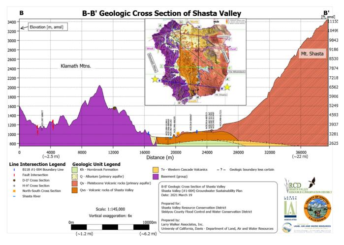
**Figure 21:** Geologic cross section B-B' from the Shasta Valley Watershed geologic model (inset includes the surface geologic overview map of the Shasta Valley Watershed geologic model.
