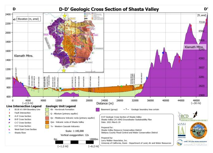
**Figure 23:** Geologic cross section D-D' from the Shasta Valley Watershed geologic model (inset includes the surface geologic overview map of the Shasta Valley Watershed geologic model.
