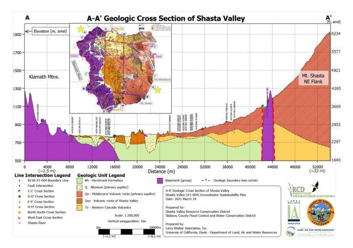
**Figure 20:** Geologic cross section A-A' from the Shasta Valley Watershed geologic model (inset includes the surface geologic overview map of the Shasta Valley Watershed geologic model.
