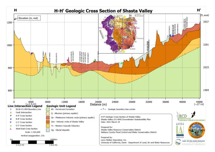
**Figure 25:** Geologic cross section H-H' from the Shasta Valley Watershed geologic model (inset includes the surface geologic overview map of the Shasta Valley Watershed geologic model.
