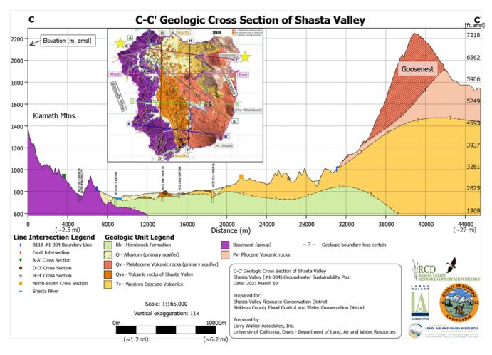
**Figure 22:** Geologic cross section C-C' from the Shasta Valley Watershed geologic model (inset includes the surface geologic overview map of the Shasta Valley Watershed geologic model.
