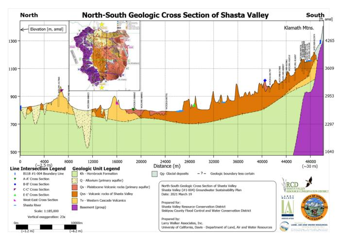
**Figure 26:** Geologic cross section North-South from the Shasta Valley Watershed geologic model (inset includes the surface geologic overview map of the Shasta Valley Watershed geologic model.
