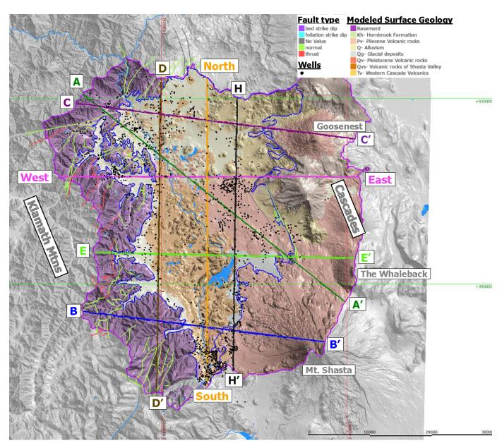
**Figure 19:** Shasta Valley Watershed geologic model overview and cross section map. Wells pictured in the map are the approximate locations noted in the Well Completion Reports used to construct the geologic model. The surface geology utilized in the geologic model is based on CDWR (2011) and SVRCD (2018).
