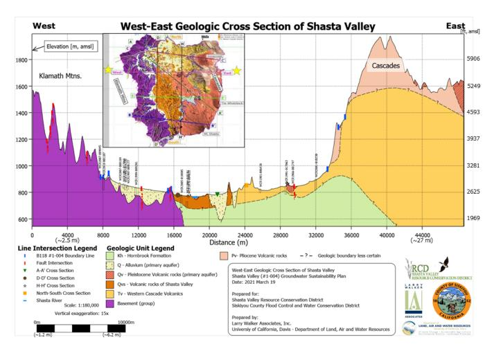
**Figure 27:** Geologic cross section West-East from the Shasta Valley Watershed geologic model (inset includes the surface geologic overview map of the Shasta Valley Watershed geologic model.
