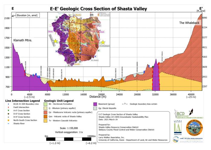
**Figure 24:** Geologic cross section E-E' from the Shasta Valley Watershed geologic model (inset includes the surface geologic overview map of the Shasta Valley Watershed geologic model.
