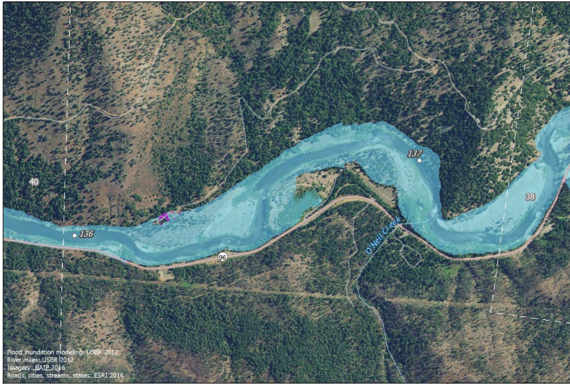
Modeled 100-year Flood Inundation Extent No Project (USBR) Proposed Project (USBR) River miles 0 200 400 Feet Map 39 of 57 Stillwater Sciences Klamath River
