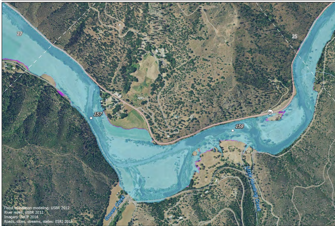
Modeled 100-year Flood Inundation Extent No Project (USBR) Proposed Project (USBR) River miles 0 200 400 Feet Map 26 of 57 Stillwater Sciences Klamath River
