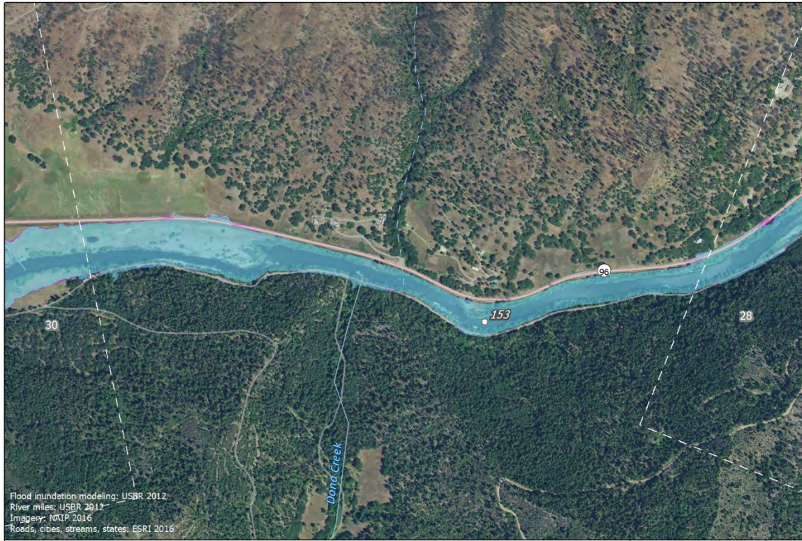
Modeled 100-year Flood Inundation Extent No Project (USBR) Proposed Project (USBR) River miles 0 200 400 Feet Map 29 of 57 Stillwater Sciences
