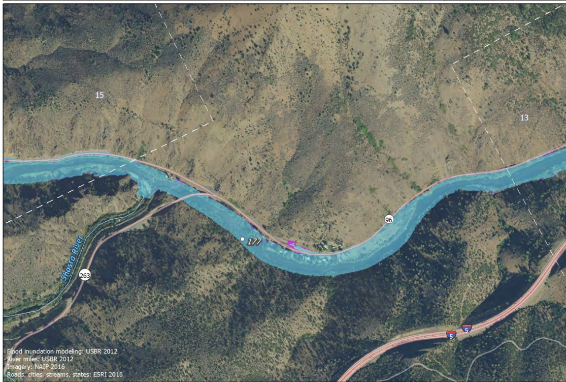
Modeled 100-year Flood Inundation Extent No Project (USBR) Proposed Project (USBR) River miles 0 200 400 Feet Map 14 of 57 Stillwater Sciences
