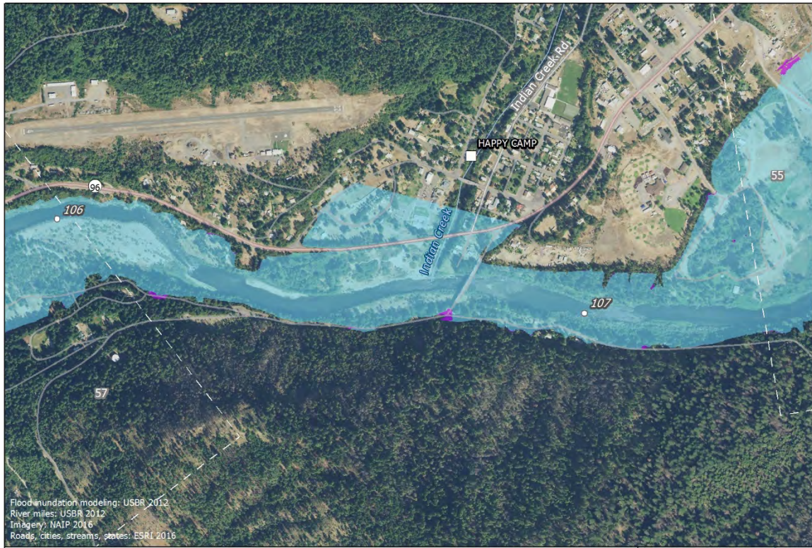
Modeled 100-year Flood Inundation Extent No Project (USBR) Proposed Project (USBR) River miles 0 200 400 Feet Map 56 of 57 Stillwater Sciences Klamath River
